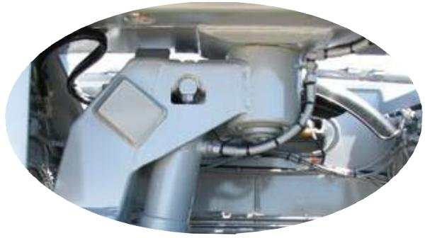
Heavy duty modular vehicles with pivot bearings are primarily intended for on-road service. On the basis of their reinforced frames, the vehicle types THP/MT and THP/ST are also well-suited for intra-plant operation at high axle loads.
