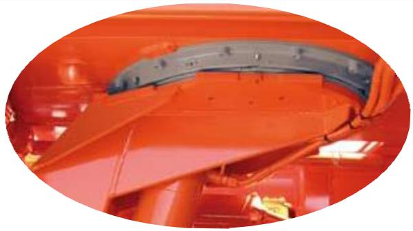
Heavy duty modular vehicles with ball-bearing race ring are specially designed for heavy loads in off-road service. The robust construction and the high bending moment guarantee safety and capability even on the most uneven terrain. The vehicle types THP/HL and THP/DL with special wheelbase have been developed for on-road service in North America.
